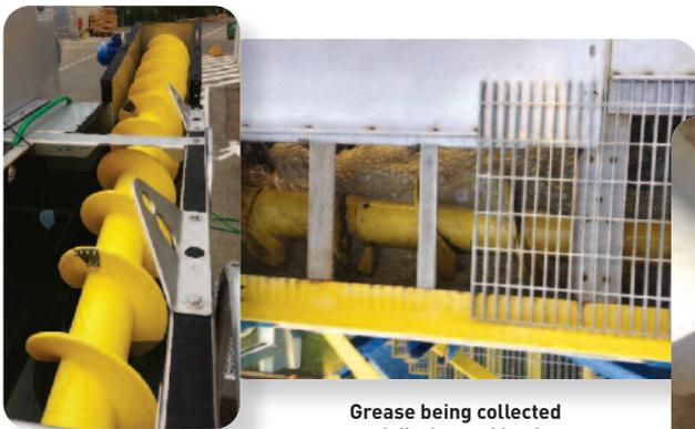
Grease being collected and discharged by the TSF floating screw.
